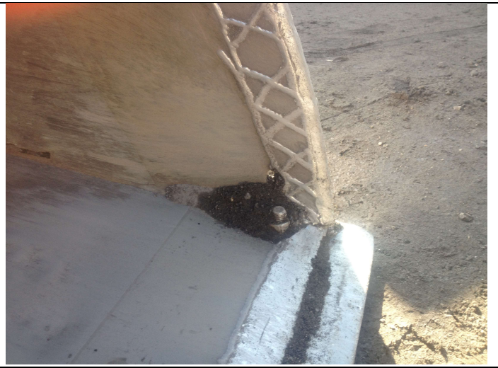
Patterns have less heat but still permit bucket wear
