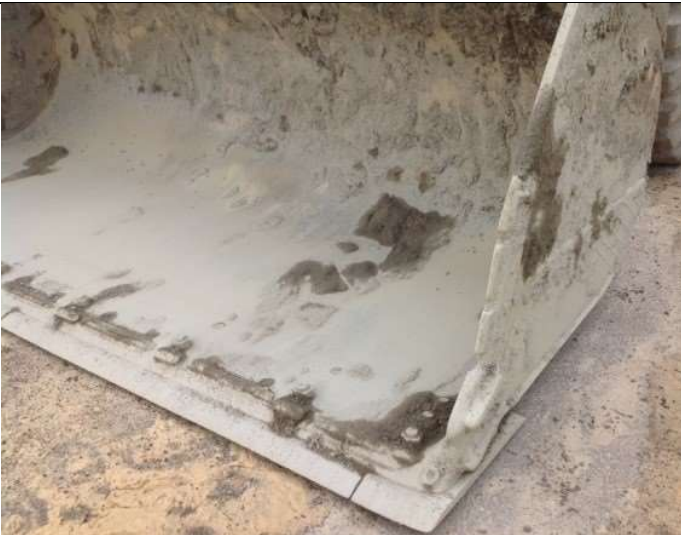
Block sections still allow bucket wear And note wear of hardsurface on sides
