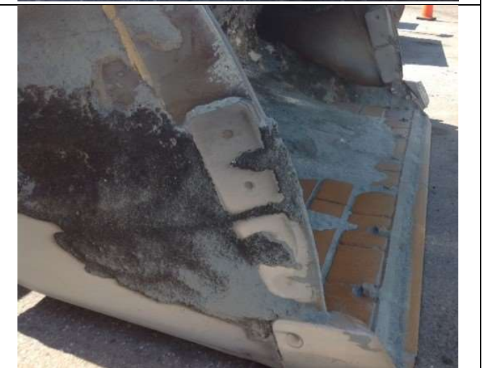
Tungsten Carbide Bevel Strip, Tungsten Carbide Vertical Side Strips, 8" X 12" Wear Patch Tungsten Carbide Corner Guards added later and inside floor replaced later (floor sizing err caused removal of one row of wear patch)
