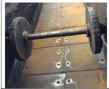
Wear plates can be replaced without breaking the slat chain
