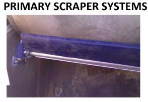
We also manufacture our own mounting systems using either spring tensioners or counterweights.
