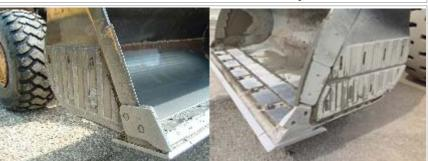
Solid 5/8" thick custom-shaped plates with overlay placed to provide strategic protection. Slotted weld holes for easy installation.
