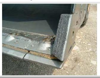
**OEM Corners Guards damage bucket before wearing out**
