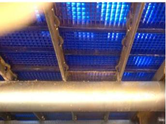
All steel stringer construction: Steel top flat welded to steel vertical flat, both with holes to permit insertion of pegs on bottom of polyurethane or rubber screen modules. Ideal for long-term maintenance. Top piece can even be used to repair competitive systems using pipe spacers. One of narrowest stringers on the market enabling highest available open area in module design.
