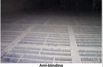
Combat blinding and get longer wear-life Works especially well on high-frequency, end-tension screens
